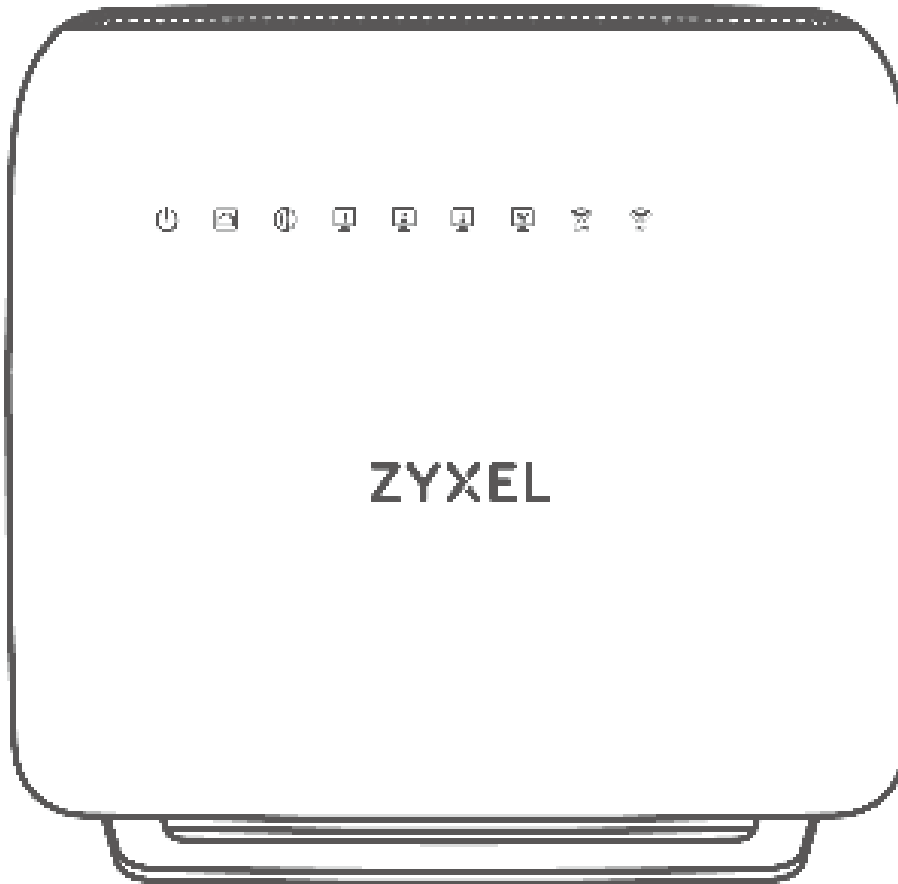
Figure 12 LED Indicators (DX3300-T1)
