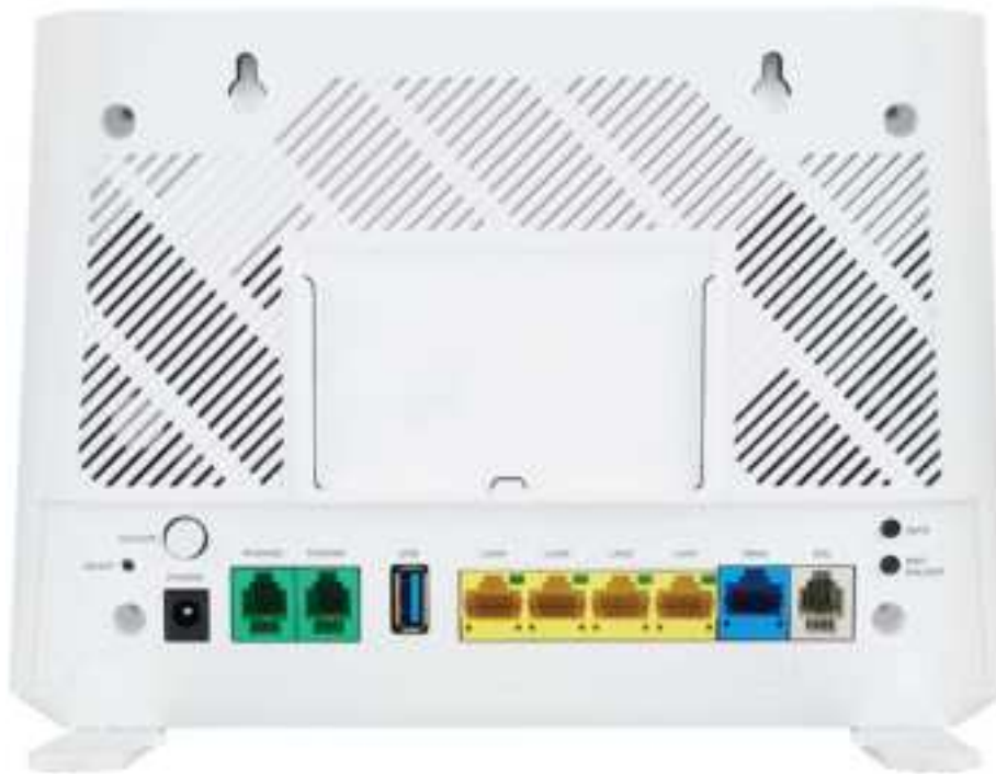
Figure 32 Rear Panel (DX3301-T0)
