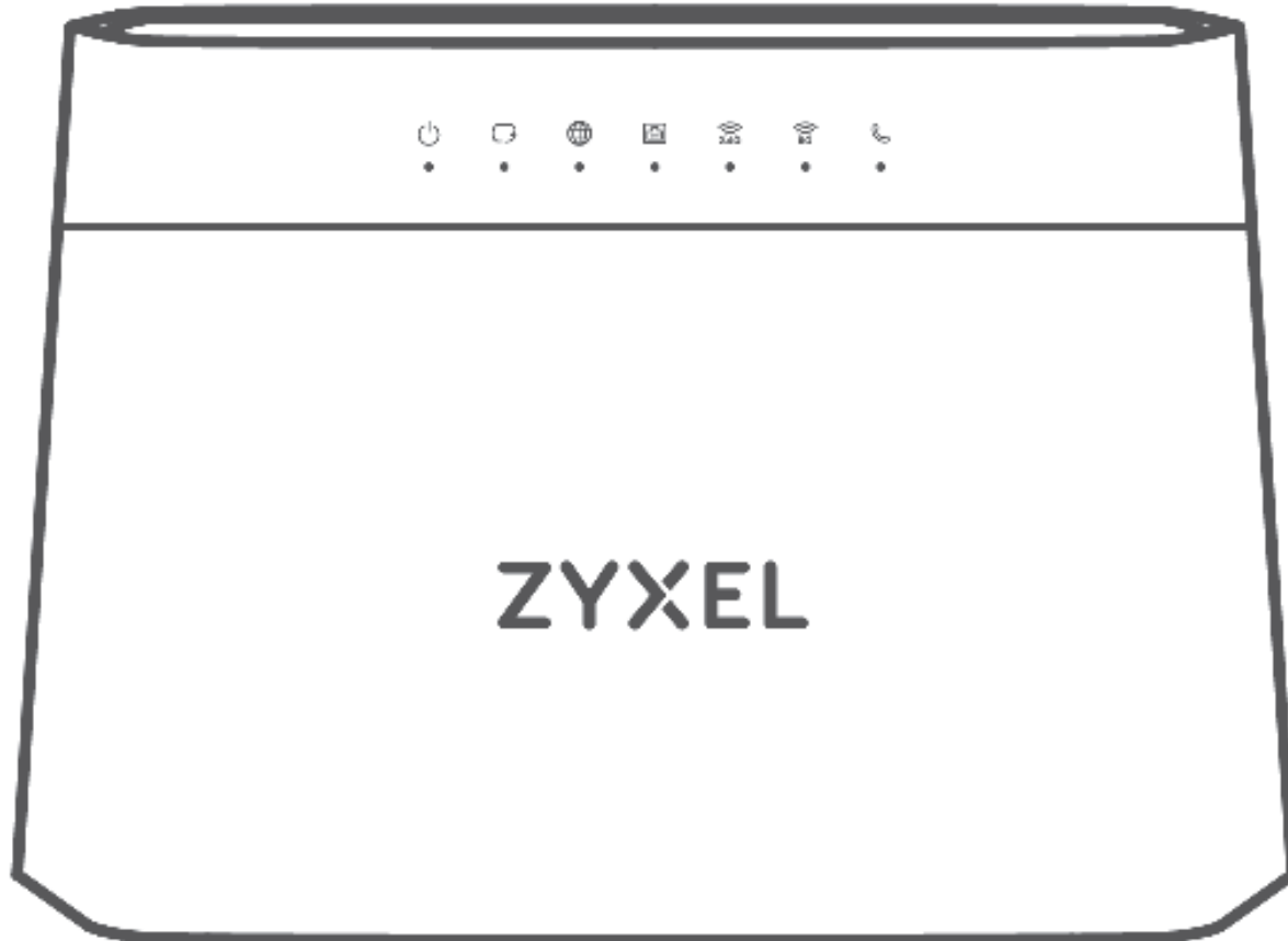
Figure 11 LED Indicators (DX3300-T0 / DX3301-T0)
