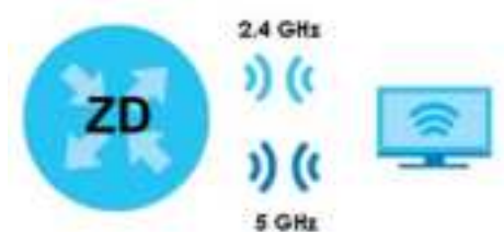
Figure 132 Multi-Link Operation Example
