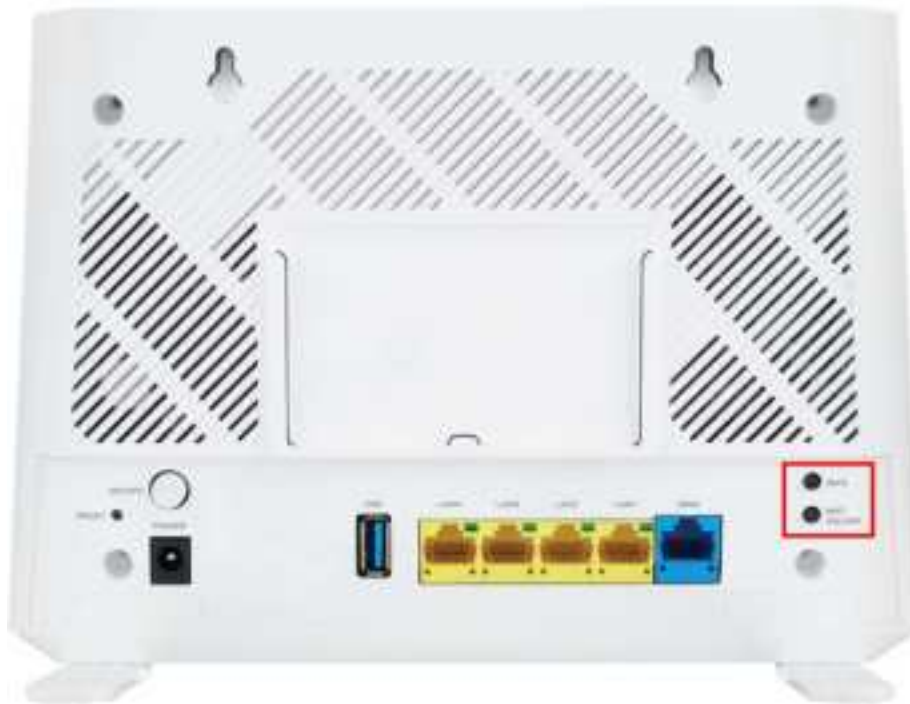
Figure 43 WPS and WiFi ON/OFF Buttons (EX3301-T0)
