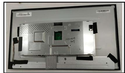
Disassembly Internal Remove All Tapes
