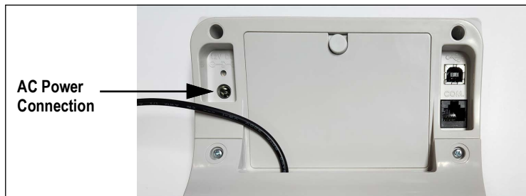
Figure 2-2. Power Connection Site
