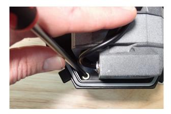
3. Place the tray slightly to the side in the housing. Keep it upright so that the bolt doesn't fall out.
