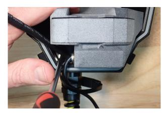
11. Before installing the camera, make sure that the inside of the domes are free from smudges and dust. Dust or dried drops of water show up very large in the 360 recording.
