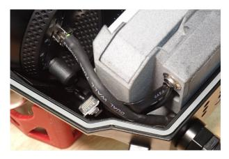
14. **Hybrid cable only**: Replace the original battery tray with the DC converter tray and connect the power lead from the hybrid bulkhead.
