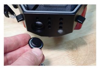
2. Remove the bolt securing the tray to the housing with a 4mm hex key or driver. You do not need to remove the bolt from the tray.
