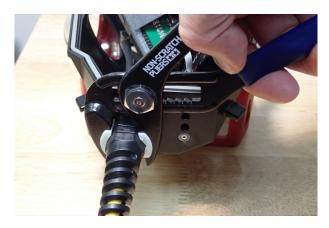
**Notes for hybrid cable installation**: The hybrid cable features a waterproof connector, which can be detached from the bulkhead. Please make sure the cable is detached from the bulkhead during installation.
