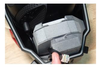
13. Now connect the newly installed cable to the camera. Fold the flat housing ethernet cable that comes with the internal tray away, it is not used in this configuration.
