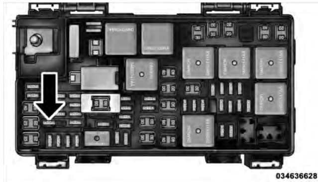
Power Outlet Fuse Location
