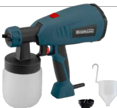
Hvlp hand held spray gun • 400W • Max Viscosity 60Din/sec • Max Water Consumption 800ml/min • Container 800ml • Including Nozzles Ø1.8/2.6mm
