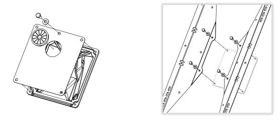
3. Place casting/bracket assembly on back surface of solar panel. Align bracket holes with solar panel frame holes and fasten as shown with included hardware: four bolts, four lock nuts and eight flat washers.
