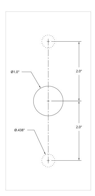
7. Band or bolt hub plate to post using suitable hardware.
