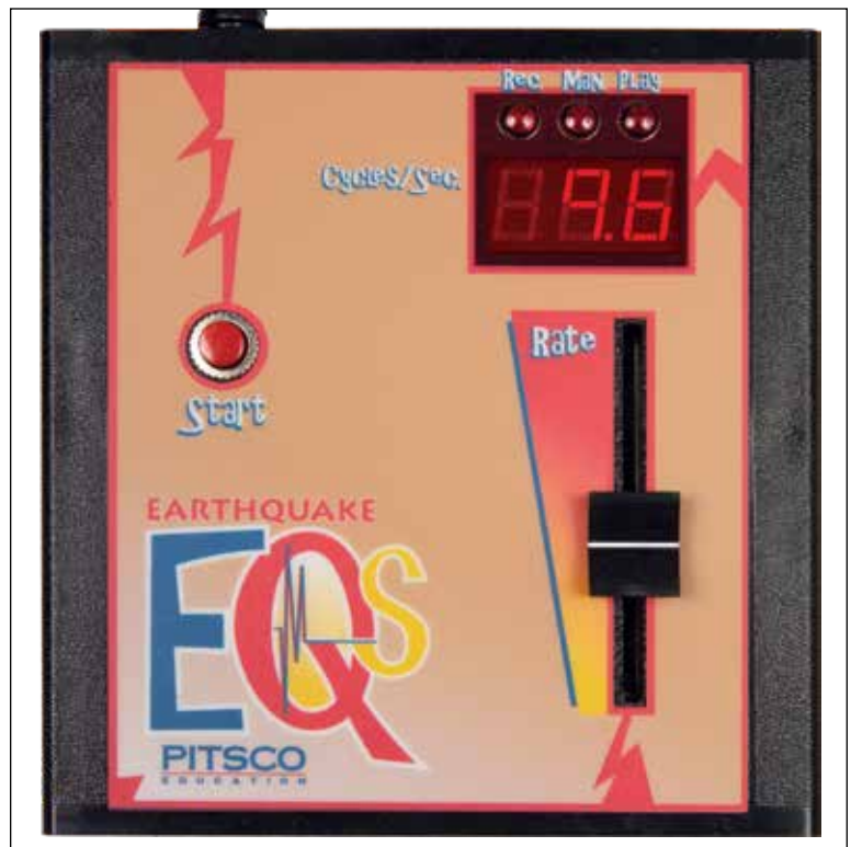
Figure 7 – Moving the Rate slide control changes the frequency.
