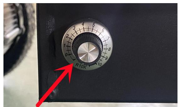
This switch is used to adjust the speed of start-up. 0 represents the slowest start-up speed and 10 represents the fastest start-up speed. Please pay attention to safety when the starting speed of the first attempt is the fastest
