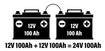
Note: If you need to connect 2 or more 12v batteries in series, please prepare a battery equalizer for balancing charge. Or you should charge them separately to avoid the voltage difference.
