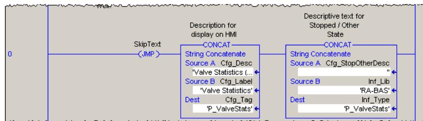
To access the valve statistics from the faceplate for the valve, you must configure MyValveMO. Set the Cfg\_HasStatsObj parameter to 1. There is no need to set a global object parameter, but the P\_ValveStats backing tag must be named the same as the Valve tag plus '\_ValveStats'.
