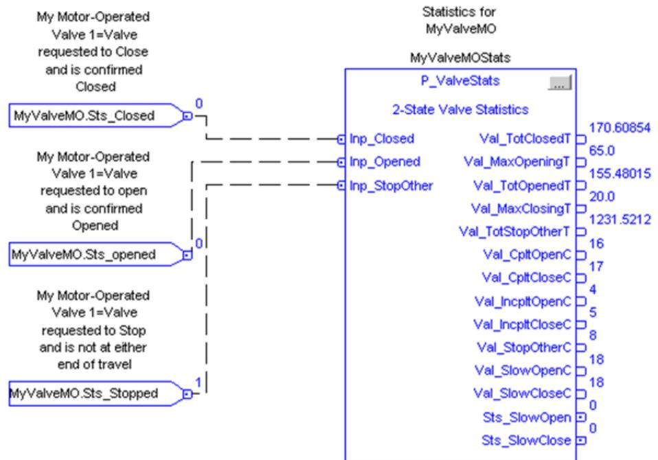
In this example, the parameters Inp\_Closed, Inp\_Opened, and Inp\_StopOther are connected to the parameters Sts\_Closed, Sts\_Opened, and Sts\_Stopped of the P\_ValveMO instruction.
