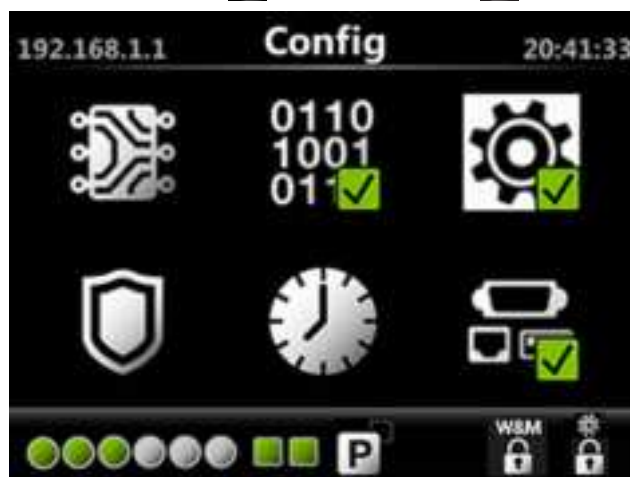
CIU 888 display: W&M relevant configuration settings are locked
