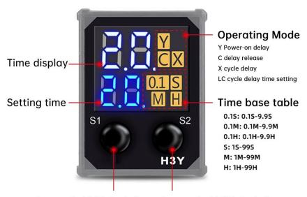
Long press the left S1 button for 3 seconds, the mode blinks and then automatically cycle switching, stop to the desired mode to release the button can be, after 5 seconds to stop blinking Long press the right S2 button for 3 seconds, the time base flashes and then automatically cycle switching, stop to the desired time base to release the button can be, 5 seconds after the automatic save.
