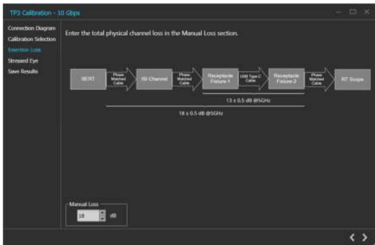
Figure 30: TP3 Calibration-Insertion Loss
