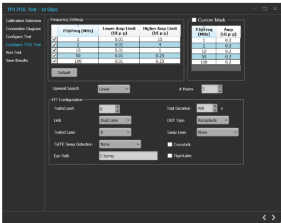
Figure 42: JTOL Test-Configure JTOL Test
