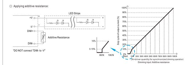
Note: 1. Min. duty cycle of output current is about 0.15%, and the dimming input is about  $6K\Omega$  or 0.6VDC, or 10V PWM signal with 6% duty cycle. 2. The duty cycle of output current could drop down to 0% when dimming input is less than  $6K\Omega$  or less than 0.6VDC, or 10V PWM signal with duty cycle less than 6%.
