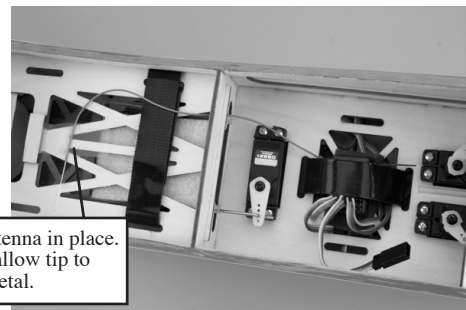
Example of AR500 installed in Hangar 9® Pulse™ XT 60
