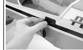
A, B. Insert bind plug into charge jack, apply power
