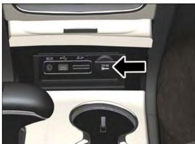
Front Power Outlet
