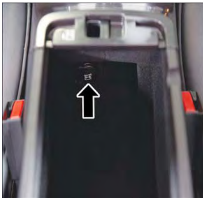
Center Console Power Outlet
