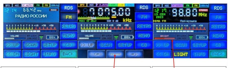
The appearance of the screen with the FM button activated. You can switch the FM band stations stored in the memory bank for the current city with the encoder.
