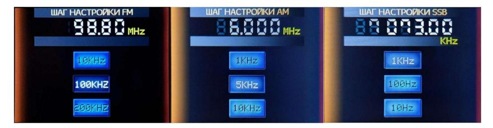
Setup step selection screens for FM - AM - SSB bands. Click the button to use the configuration step indicated on it.
