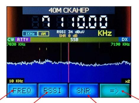
A button to change the scale of the graph in the frequency domain (X-axis). Adjustment using an encoder
