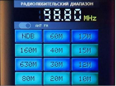
A screen for selecting the broadcast range, with an indication at the top of the currently used frequency.
