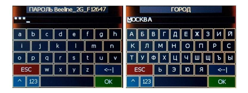
This on-screen keyboard appears when it is necessary to enter characters and data on the receiver pages, the password of the Wi-Fi access point, the firmware activation key, editing the names of memory stations, cities... and much more. Use the "^" and "123" buttons to activate uppercase/lowercase/numeric/special characters. OK to confirm. ESC to cancel.
