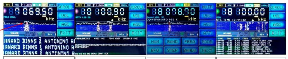
The FELD-HELL digital mode decoding screen ("Minifax"). To shift the image vertically, press SCROLL and rotate the encoder. Press EXIT to exit the decoding mode.
