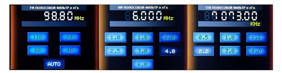
Screens for selecting the bandwidth used (bandpass filter) for FM – AM – SSB with an indication of the current filter.
