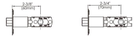
Measure distance between the center of the hole to the edge of door, adjust latch F to 2-3/8"(60mm) or 2-3/4"(70mm)
