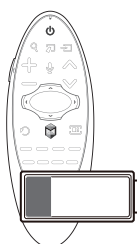
<Low battery Alarm Icon>
