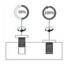
Before the complete installation, do not tighten the screws all the way. You can first tighten the screws to 50%, and then once the entire assembly is complete, you can fully tighten all the screws
