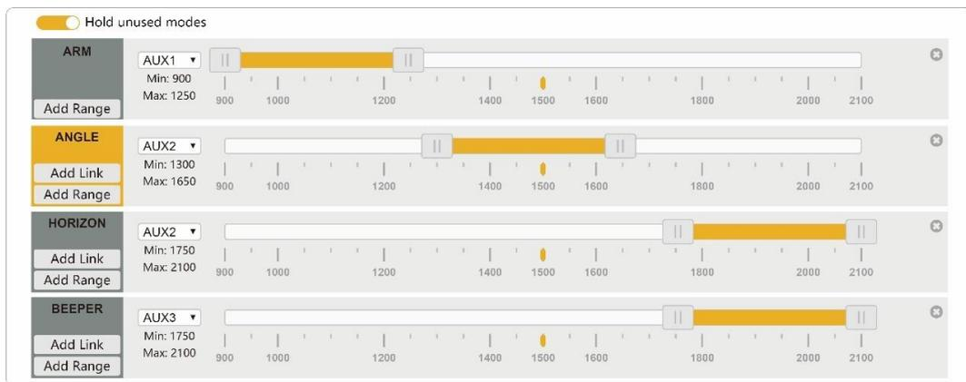
2. DJI toggle switches are all three sections. If you move the Yellow cursor of the corresponding aux channel of the switch, the corresponding function will be turned on when you move to the set range.
