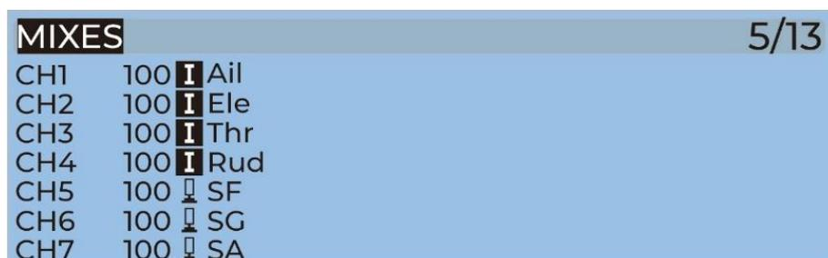
2. FrSky X9D transmitter SF toggle switch are two sections. If you move the Yellow cursor of the corresponding aux channel of the switch, the corresponding function will be turned on when you move to the set range.
