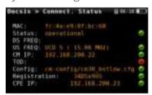
Obtain a step-by-step indication of a Pass/Fail test, as the modem finds, connects, and registers to a headend (CMTS), and also obtains critical parameters in the process. Confirm that the modem first finds the downstream channel and, right after that, the upstream channel. Later obtain the configuration as the DHCP address server, TOD server time, the complete configuration file and the registration information.
