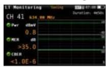
This H30D+ Long Term Monitoring Function allows the automatic monitoring of the selected channel. Once the time interval between two consecutive measurements has been selected, the H30D+ will automatically take all the measurements of the channel selected and store them in memory.
