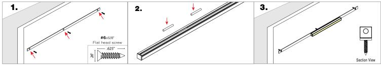
Using the #6 Flat head screws, mount screws into the magnet bracket through the drilled holes.
