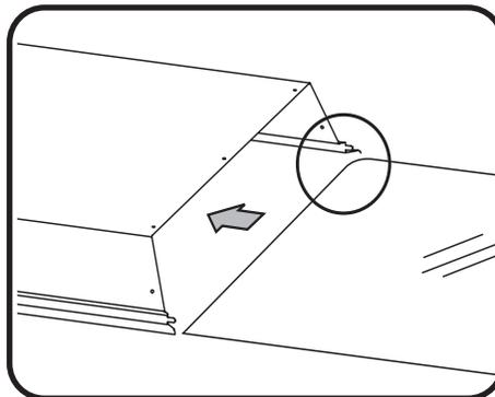
**5** Slide in the new diffuser. Make sure the round corner on the diffuser slides in first as shown in the circled area of the above picture.
