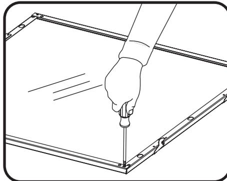
5 Reattach end rail with screws.
