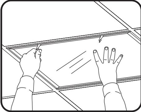
1 Rotate latches to unlock the front bezel.
