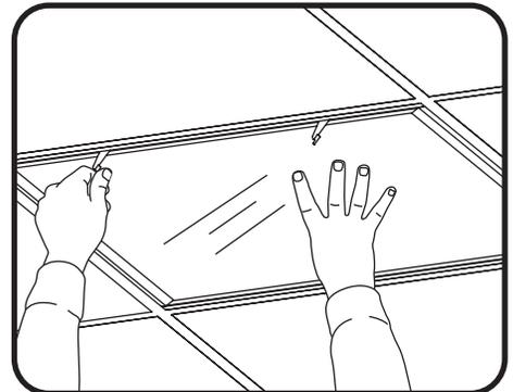
6 Hang panel on its hinges and swing up into place. Rotate latches on front bezel to fasten it.
