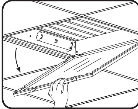
2 Swing down panel and lift off front bezel with diffuser.
