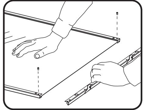
3 Place front bezel with diffuser on table. Unfasten the two rail screws on the end rail with latches, then remove this end rail.
