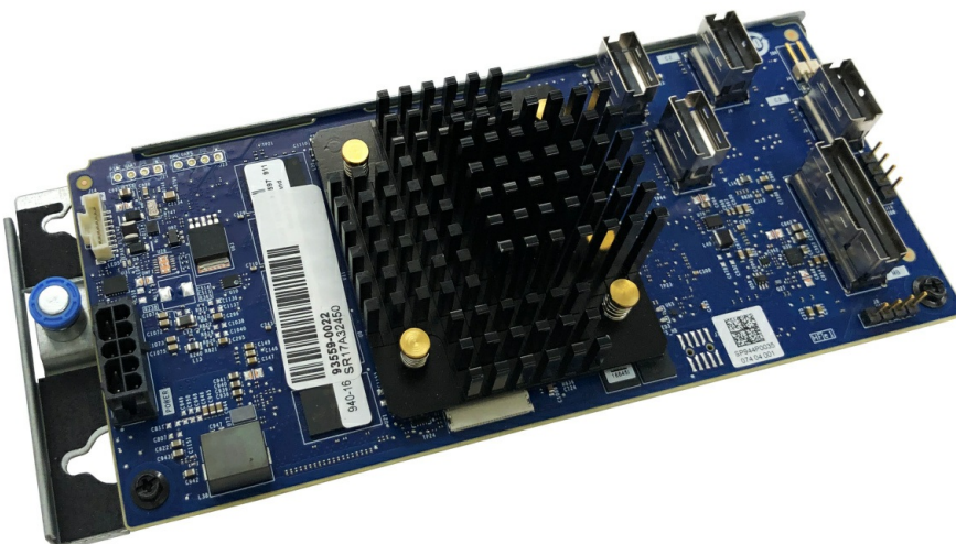
Figure 3. ThinkSystem RAID 940-16i 8GB Flash PCIe Gen4 12Gb Internal Adapter
