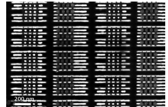
FinFET transistor, top view, 22 nm technology, 3 kV, pure BSE imaging using Inlens EsB, high material contrast.
