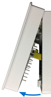
Illustration 4—Removing the Cover from the Backplate
