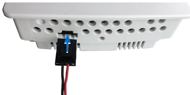
Illustration 14—MS/TP (EIA-485) Data Port
