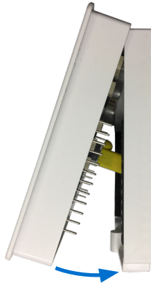
Illustration 7—Reinstalling the Cover on the Backplate
