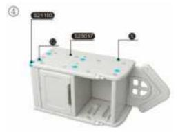
Fasten and tighten the nut, and cover the Cover the S23017 storage side panels with Z2 large cross nuts and X small crosses fillet buckle.
