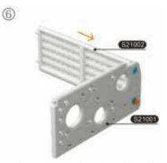
Insert the long layer board into the two holes on the top of the storage side panel, and fix it with the Z2large cross nut.
