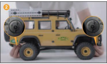
转动前后快拆旋钮,听到明显的卡扣声标志车身已经打开 Twist the quick release tabs to detach the vehicle body from the chassis. An audible click will confirm the body is securely opened.
