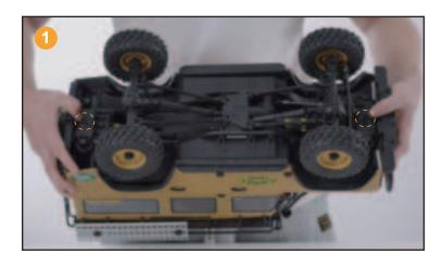
快拆底部前后旋钮 Locate the quick release tabs as shown in the diagram above.
