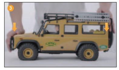
前后同时按压车身,有明显的卡扣闭合声音;车壳即安装完成 Simultaneously press down on the front and rear of the body. An audible click will confirm the body is securely attached.
