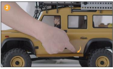
车身放置于脚踏板内侧 Align the vehicle body with the chassis' running boards.
