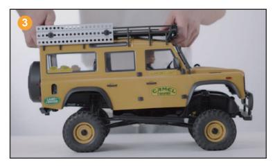
取下车壳 Remove the vehicle body.
