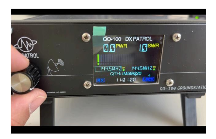
Showing also the TX and RX band IFs ON or OFF, UTC clock, Locator and Locking to GPD Wait or Lock.
