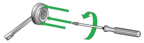
3. Gently remove the battery and replace it with the new one.
