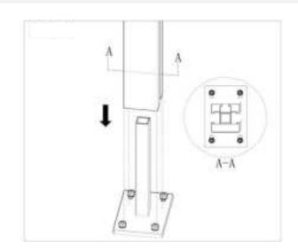
With the screws provided (A4), screw in the board stopper through both the post and fixing post support (Figure B-B). The board stopper on your post may come pre-installed. If this is the case, uninstall the board stopper before installing onto the fixing post support.
