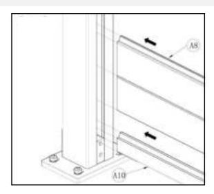
Then, slide the boards (A8) into the slots of the post. Each board should nest into the one below it. When installing the boards, it is necessary to leave a gap of 9mm | 0.3 inches between the fence board and the center rib of the posts on each side (see the figure on right).
