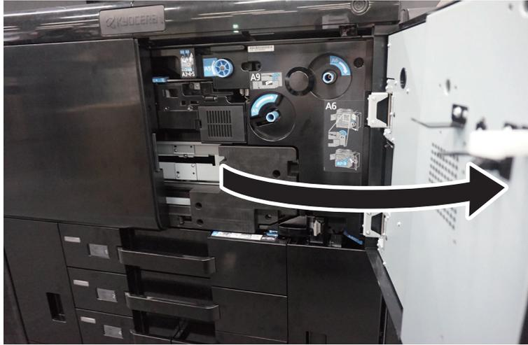
When adjusting the feeding pressure of the cassette 4, also open the front cover 4. This makes it easier to operate the paper feed pressure dial.
