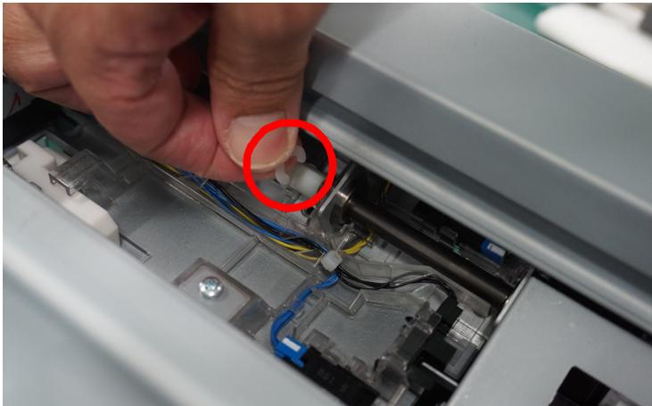
**22 Move the pickup adjustment lever to its original position.**
