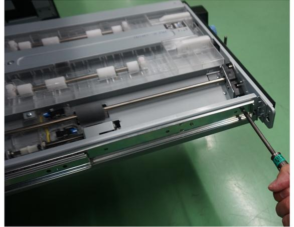
**10 Remove the deck feed unit in the direction of the arrow.**
