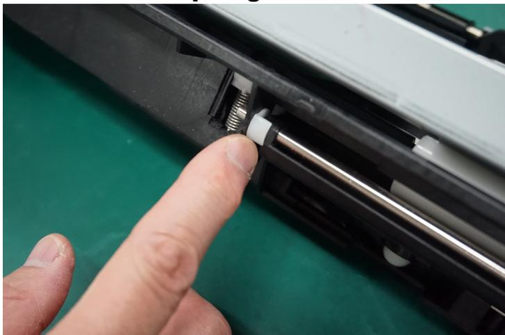
**13** Pull out the shaft in the direction of the arrow.
