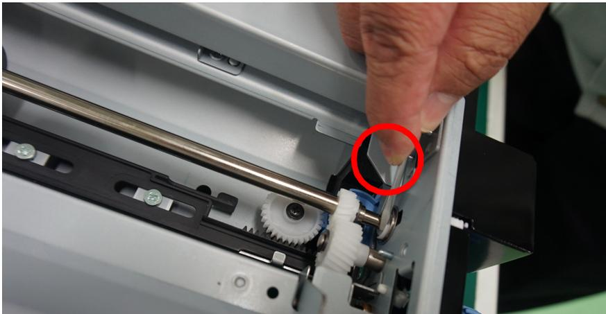
**14 Remove the transfer roller in the direction of the arrow.**
