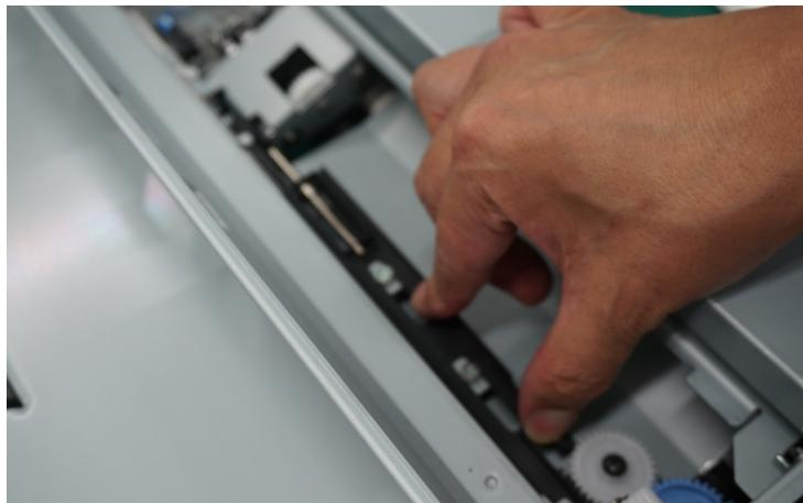
**19 Attach the horizontal conveying upper guide, and then the stop ring.**
