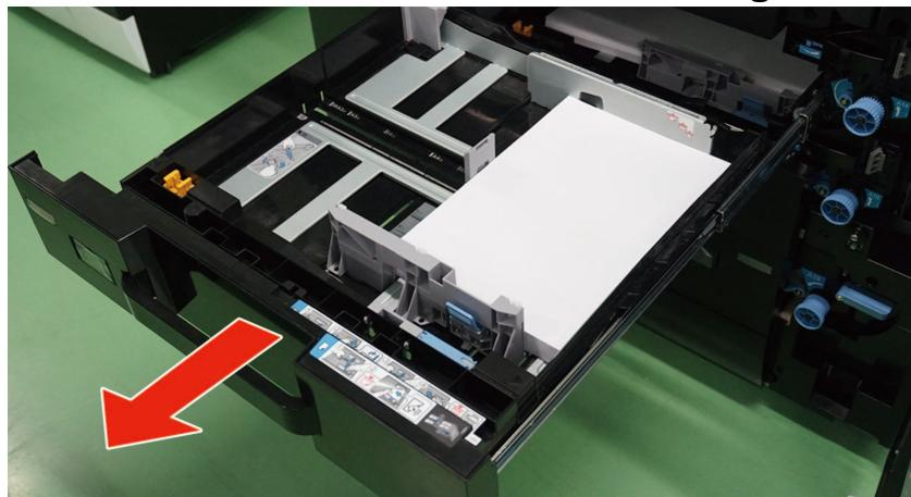
**4 Move the lock lever to the arrow direction to release it and pull out the cassette feed unit.**
