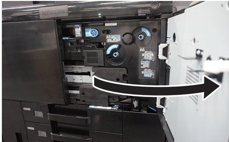
When adjusting the feeding pressure of the cassette 4, also open the front cover 4. This makes it easier to operate the paper feed pressure lever.
