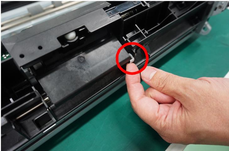
**23** Pull out the shaft in the direction of the arrow.
