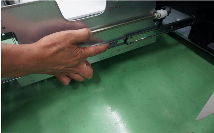
**7 Turn the lever until it stops to release the lock.**
