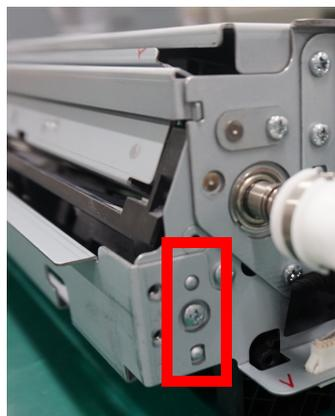
**37 Attach the feed roller drive assy.**
