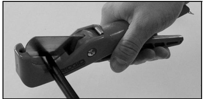
Figure 84: Cutting the Cable
