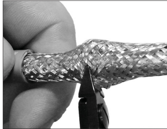
Figure 34: Cutting the Cable Braid Bulge
