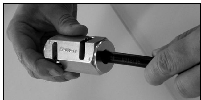
Figure 87: Stripping the End to Expose the Center Conductor
