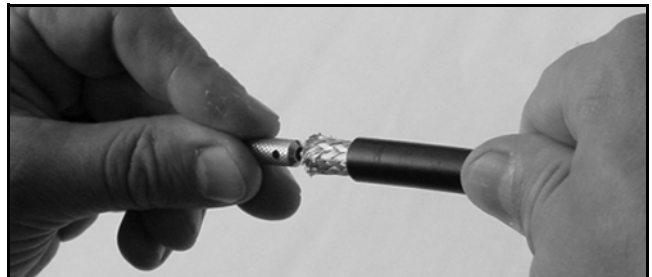
Figure 91: Deburring the Center Conductor
