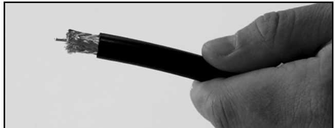
Figure 90: Cable Stripped, Exposing Dielectric
