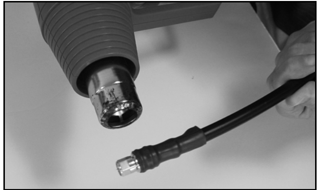
Figure 97: Applying the Heat Shrink Tubing
