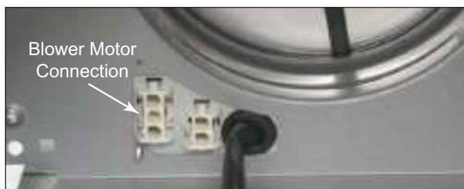
Figure 4-10. Blower Connection in Easy Cube
