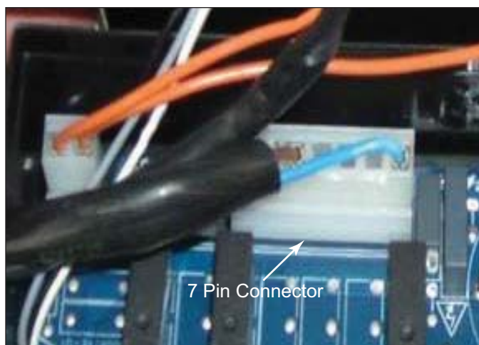
Figure 4-3. 7 Pin Connector in Power Board
