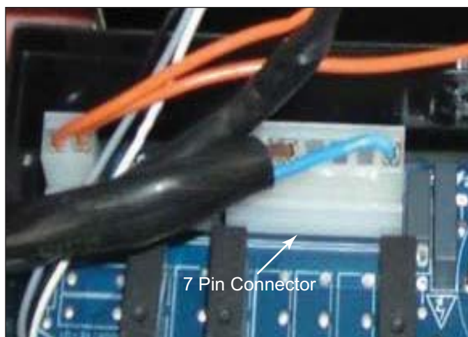
Figure 4-3. 7 Pin Connector in Power Board
