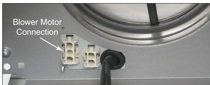
Figure 4-10. Blower Connection in Easy Cube
