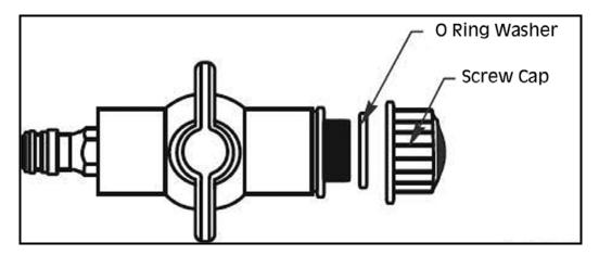
2. Place the main body of the outlet/drain tap through the outlet holes in the tank exterior and replace the O ring and filter screw cap on the inside of the water tank, as shown.
