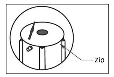
The lid has a polyester/PVC mesh filter in the centre to stop large impurities such as leaves entering the tank.
