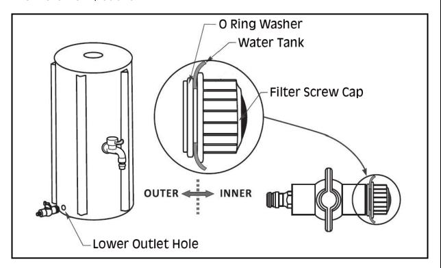
3. Take the overflow pipe and unscrew the filter screw cap.
