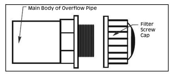
4. Place the main body of the overflow pipe through the outlet hole in the tank exterior and replace the filter screw cap on the inside of the water tank, as shown.
