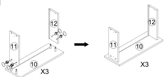
When installing No. 10, No. 11, No. 12, if the B screw cannot be tightened, please rotate the A screw on No. 10 counterclockwise 90-120 degrees, and then tighten the B screw.
