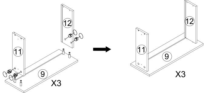
When installing No. 9, No. 11, No. 12, if the B screw cannot be tightened, please rotate the A screw on No. 9 counterclockwise 90-120 degrees, and then tighten the B screw.
