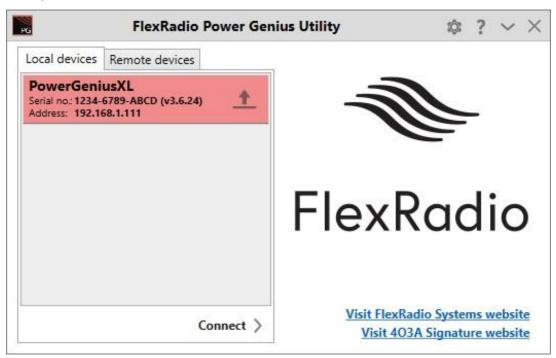
Caution: Never run earlier versions of the Power Genius Utility with new Power Genius XL firmware. Before installing the latest release of the Power Genius Utility, you should remove any earlier versions of the Power Genius Utility from all PCs on your network. This includes version v2.2.10 and below. Connecting an older version of the Power Genius Utility to a Power Genius XL amplifier can result in unexpected and unreliable behavior.
