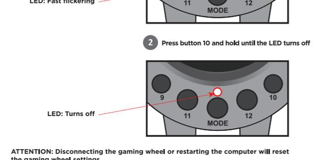
**ATTENTION: Disconnecting the gaming wheel or restarting the computer will reset the gaming wheel settings**
