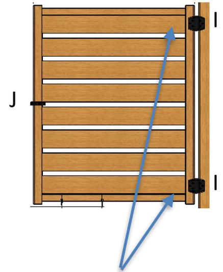
Hinges position should be installed as shown in drawing [2.5 inches from the top and bottom]
