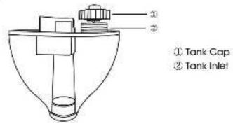
Rotate the cap in the "open" direction to remove the cap, add an appropriate amount of water into the tank, and screw the cap back on in the lock direction until no water leaks. Do not rotate it with excessive force
