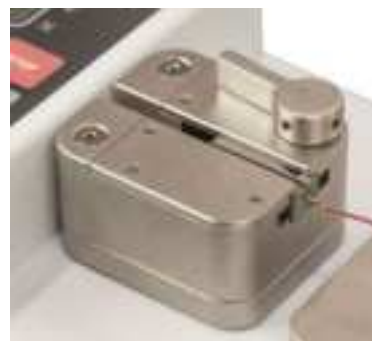
Fig. 3.3 Wedge grip assembly (optional)
