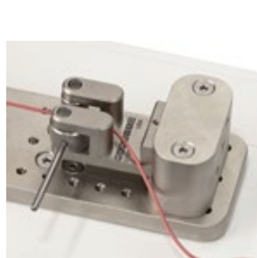
Fig. 3.6 Dual roller grip assembly (optional)
