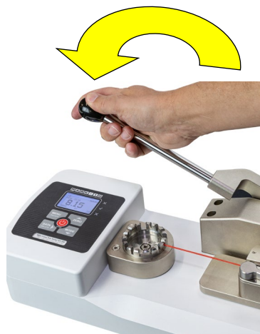
Fig. 3.7 Rotating the lever
