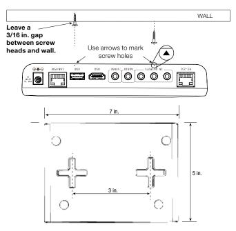
Structured Wiring Cabinet Mounting: Using the optional Structured Wiring Cabinet Mount, the EL-SC-100 can be mounted in a structured wiring cabinet.
