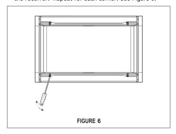
4. BACK FRAME INSTALLATION: Position BACK FRAME with equal space top to bottom, side to side. Mark for 4 holes, center punch and pre-drill the cabinet with 1/16" drill bit. Secure frame with 4 SCREWS E. See Figure 7.
