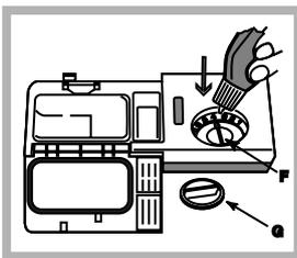
1. Open the dispenser by turning the lid (G) in an anticlockwise direction.
