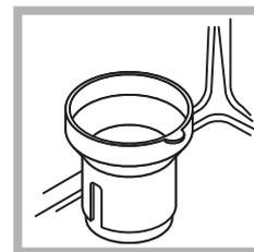
1. Remove the lower rack and unscrew the container cap (anticlockwise).
