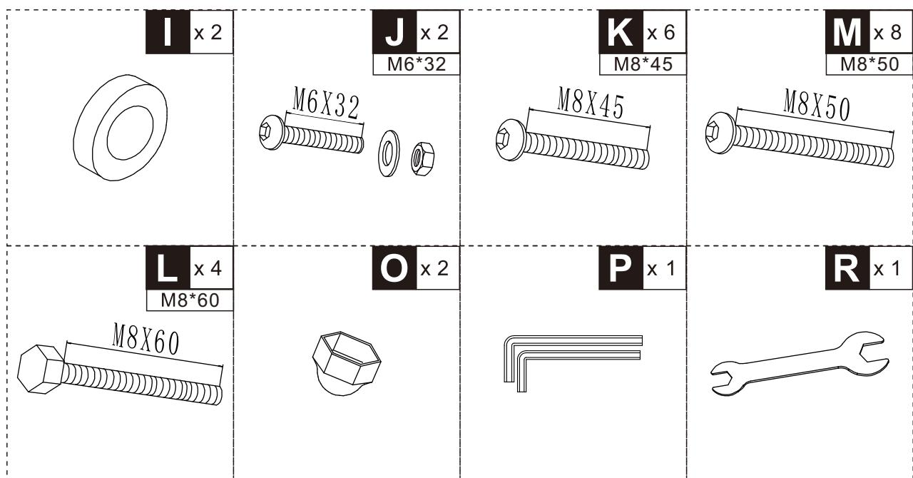
**EN** Do not tighten bolts fully until all parts are connected!
