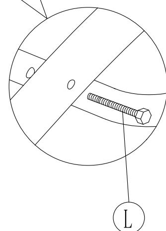
EN\_Tighten the screws on one side to 30% and then 30% on the other side and then tighten them at the same time.
